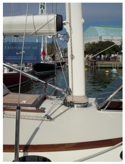
Stainless steel hydraulic vang, in-boom main furler, and mast collar with custom built-in stainless steel turning blocks.
